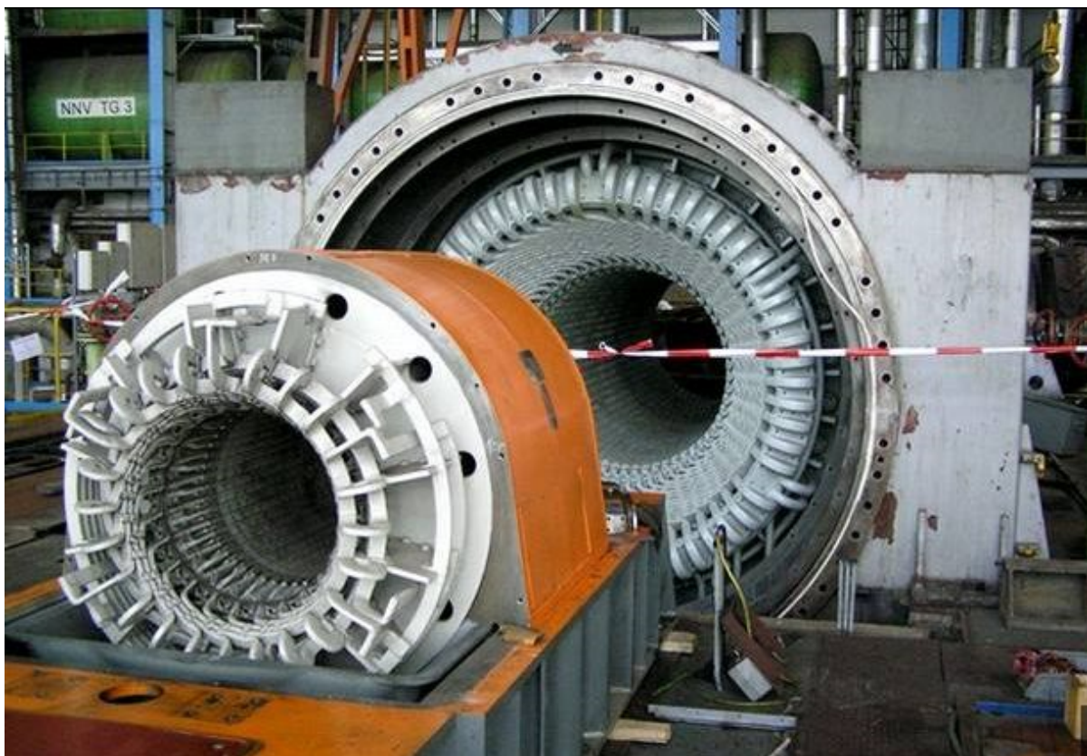
Fig. 6.4 Stator of turboalternator and its exciter (Dětmarovice power plant)
