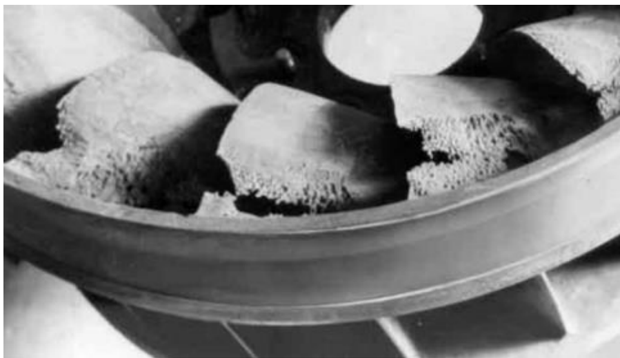
Fig. 4.10 Cavitation on the impeller of the Francis turbine
