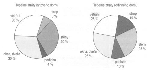
Fig. 16.3 Contribution of different structures to the heat loss of the house
